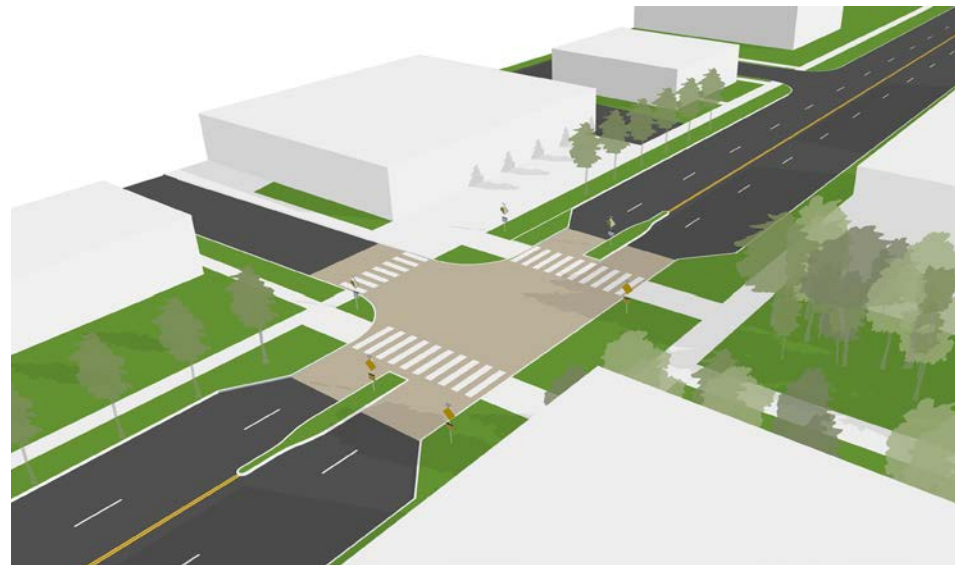
ALTERNATIVE 3 Enhanced crosswalks with pedestrian refuge islands, speed table and planted bump-outs
