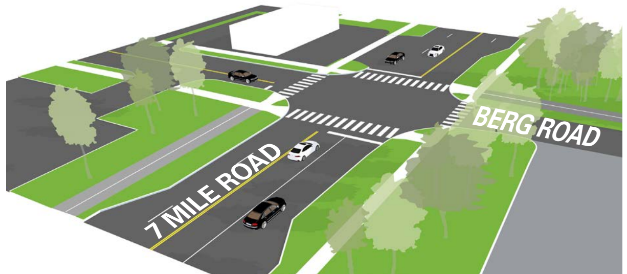
BERG ROAD AND 7 MILE ROAD INTERSECTION - PROPOSED Enhanced crosswalks and planted bump-outs.
