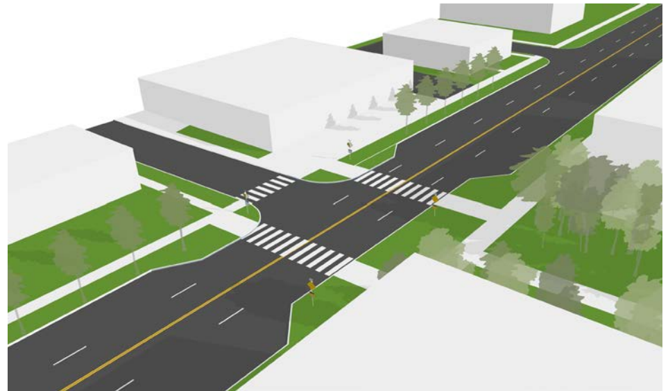
ALTERNATIVE 1 Enhanced crosswalks and planted bump-outs
